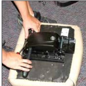
6. With all Phillips screws revealed, and removed, the mechanism can now be lifted off the seat
