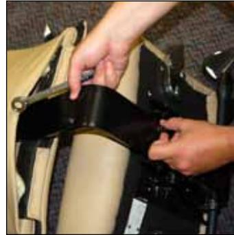
3. With the nuts removed, hold the back support steady with one hand, and push the bolts up and out of the back post, allowing the back post to slide out.
