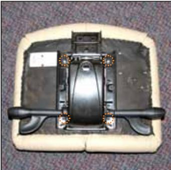
5. Locate the 4 Phillips screws securing seat to mechanism. NOTE: 2 screws may be obscured by the slider. Before releasing and moving slider to reveal them, keep hands and fingers away from the slider. The slider control is the left-side wing on mechanism.
