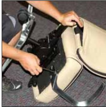
9. Reattach armrests, reinsert cylinder, and then reattach base.
