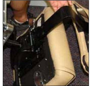
4. Position the new back for installation and reinsert the 3 bolts to hold it in place.
