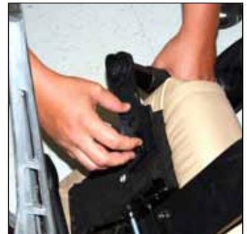
4. Set the armrest width as desired and firmly tighten the hand wheel.
