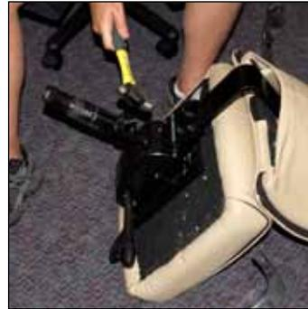
3. Hold the end of the cylinder with one hand, and hammer the mechanism around the cylinder entry point. \*\* Several strong blows may be required to dislodge the cylinder from mechanism.
