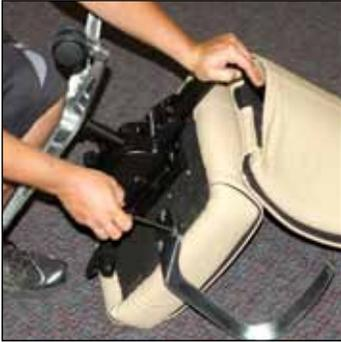
1. Remove the armrests from the chair (Reference to *Arm Replacement* sheet.) mechanism, and set aside for later reinstallation.
