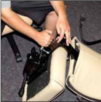
8. Reattach backrest with the 3 bolts and nuts, replacing the plastic cover (Reference *Backrest Replacement* sheet).
