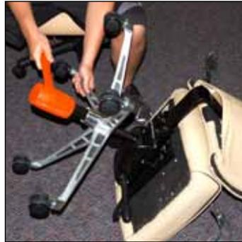
2. Tip the chair forward/over until the base is off the floor. Hold one leg of the base and strike the cylinder protruding through the base, using a plastic hammer. The force will dislodge the base.\*
