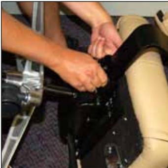
5. Replace the nuts on the 3 bolts, and gradually tighten each in rotation so all are equally set. Replace plastic cover (from Step 1).
